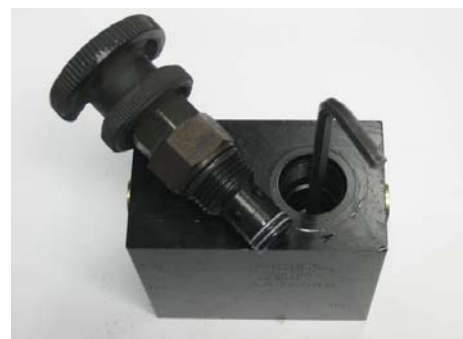
Remove the hand valve assembly with a 1” wrench to gain access to the orifice which is removed with a 3/16” Allen wrench.
